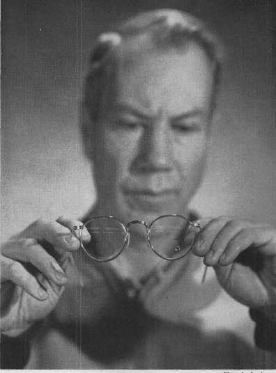
A TINY SPOT of solder on these safety glasses is inspected by Clifford C. Savage, 2122-1. Cliff's eye was probably saved by his glasses. Solder melts at about 500 degrees—hot enough to cause painful, serious injuries.
